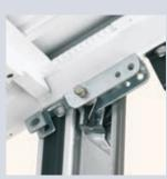
Anti-drop device to prevent the door from crashing down in the event of a spring or cable failure.
